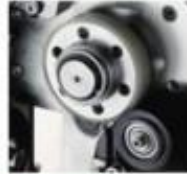
Main roller tensioning system
