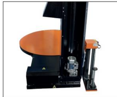
RACK AND PINION SYSTEM
